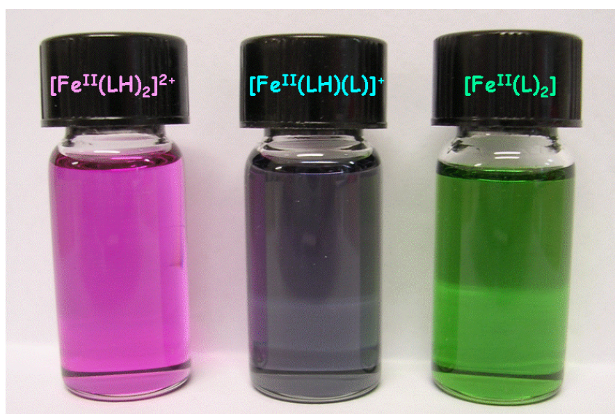
Figure S3. Colours of \text{CHCl}_3 solution 5 \times 10^{-5} M of [\text{Fe}^{\text{II}}(\text{LH})_2]^{2+} complex after the addition of 0, 1, 2 equiv. of Proton Sponge ® , 13 (from left); LH = 3 .
